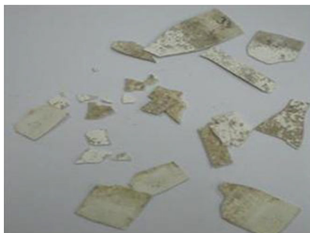
Figure 1. CS disintegrated after 2 months of weathering. [Color figure can be viewed in the online issue, which is available at wileyonlinelibrary.com .]
